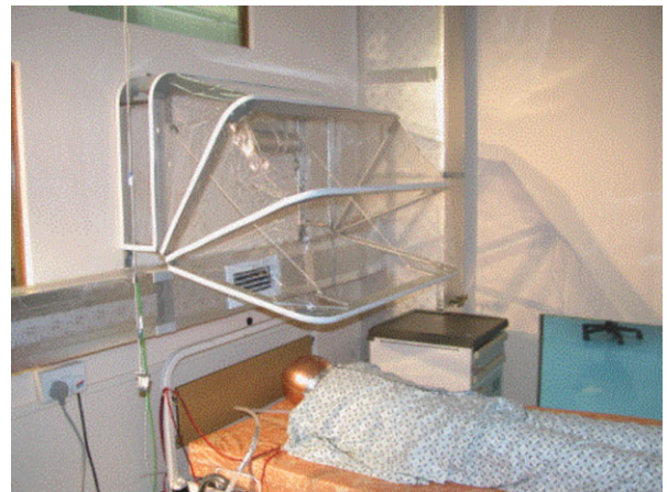
Figure 9. Retractable hood design. Idea of Victor Cheung, JRP, Hong Kong.
