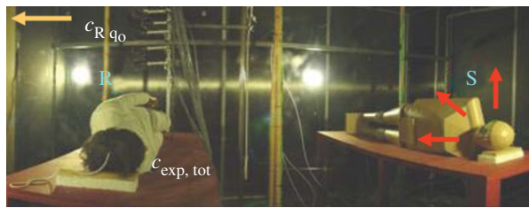
Figure 1. Two patients (life-size manikins) in a hospital ward. One patient is the source of airborne infection, and the other patient is the target.
